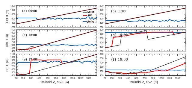
**Figure 6.** The CBL tops identified from the idealized backscatter method (*fitting*), Haar wavelet method (HM), and Mexican Hat wavelet method (MHM) with different initial values of  $z_m$  or  $\Delta h$  being set for the real profiles at (a) 09:00, (b) 11:00, (c) 13:00, (d) 15:00, (e) 17:00, and (f) 19:00 local time on 19 December 2007.
