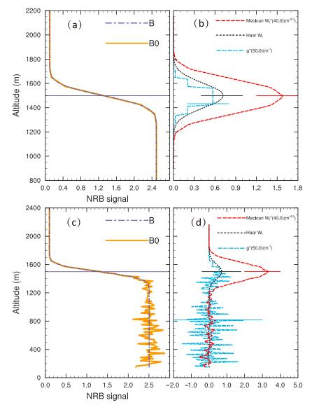
**Figure 1.** (a) The idealized profile and (c) the simulated real profile of the normalized relative backscatter signal (NRB) (B0) along with the fitted curve B, and (b and d) the corresponding profiles of gradient g, the Haar wavelet coefficient (Haar  $W_f$ ), and the Mexican Hat wavelet coefficient (Mexican  $W_f$ ). The CBL tops identified from those profiles are marked by the horizontal lines.
