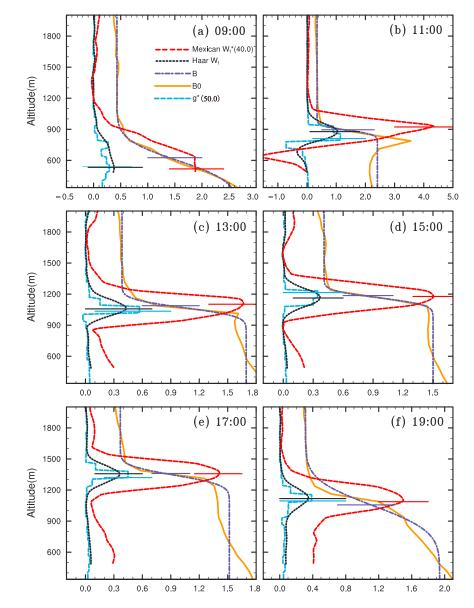
**Figure 5.** The real profile of the normalized relative backscatter signal (*B*0) with the corresponding profiles of gradient (*g*), Haar wavelet coefficient (Haar  $W_f$ ), Mexican Hat wavelet coefficient (Mexican  $W_f$ ), and fitted profile (*B*) at (a) 09:00, (b) 11:00, (c) 13:00, (d) 15:00, (e) 17:00, and (f) 19:00 local time on 16 July 2007. The CBL tops identified from those profiles are marked by the horizontal lines.
