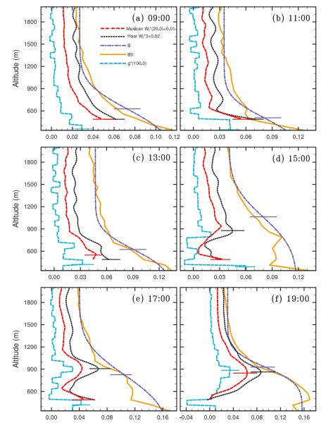
**Figure 4.** The real profile of the normalized relative backscatter signal (B0) with the corresponding profiles of gradient (g), Haar wavelet coefficient (Haar  $W_f$ ), Mexican Hat wavelet coefficient (Mexican  $W_f$ ), and fitted profile (B) at (a) 09:00, (b) 11:00, (c) 13:00, (d) 15:00, (e) 17:00, and (f) 19:00 local time on 19 December 2007. The CBL tops identified from those profiles are marked by the horizontal lines.
