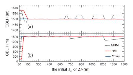
**Figure 2.** The CBLH calculated by using the idealized backscatter method (*fitting*), Haar wavelet method (HM), and Mexican Hat method (MHM) with different initial values of  $z_m$  or  $\Delta h$  set for (a) the idealized profile and (b) the simulated real profile.
