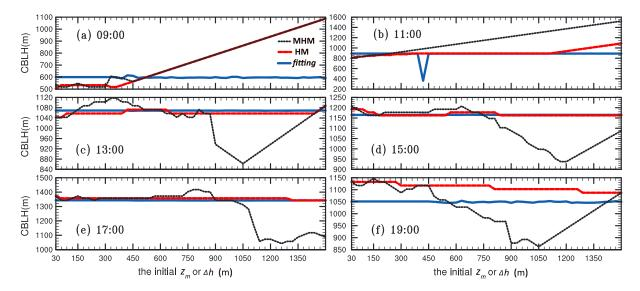
**Figure 7.** The CBL tops identified from the idealized backscatter method (*fitting*), Haar wavelet method (HM), and Mexican Hat method (MHM) with different initial values of  $z_m$  or  $\Delta h$  being set for the real profiles at (a) 09:00, (b) 11:00, (c) 13:00, (d) 15:00, (e) 17:00, and (f) 19:00 local time on 16 July 2007.
