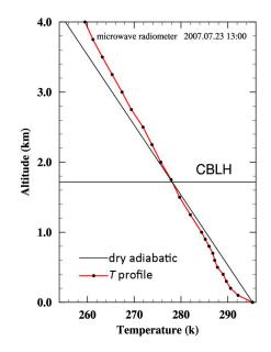
**Figure 4.** Convective boundary layer height (CBLH) determined by the parcel method applied to the microwave radiometer *T* profile. The profile is measured at 13:00 local time on 23 July 2007 at SACOL (the Semi-arid Climate Observatory and Laboratory of Lanzhou University).
