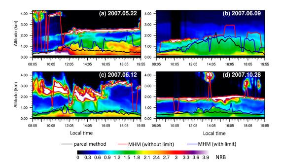
**Figure 9.** Time–height diagram of NRB (averaged every 11 min) on (a) 22 May; (b) 9 June; (c) 12 June; and (d) 28 October 2007. The CBLH calculated by the Mexican hat wavelet method (MHM) with (or without) the calculated CCL as an upper limit is marked by blue solid lines (or red solid lines), and the  $\Delta h$  used by the HM is set to 300 m based on the previous sensitivity test. The CBLH estimated by the parcel method is marked by black solid lines.
