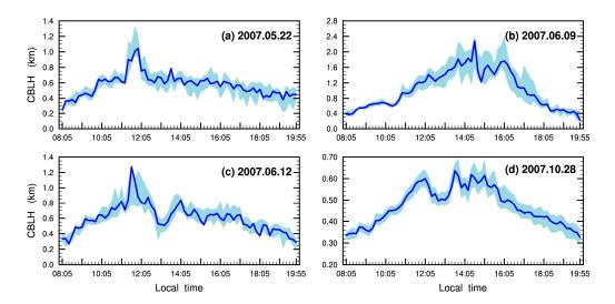
**Figure 6.** The CBLH values calculated by the parcel method on (**a**) 22 May; (**b**) 9 June; (**c**) 12 June; and (**d**) 28 October 2007 (blue solid lines). The shaded area in light blue in each plot represents the uncertainties in the CBLH caused by the surface temperature.
