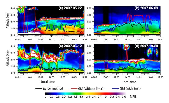
**Figure 10.** Time–height diagram of NRB (averaged every 11 min) on (**a**) 22 May; (**b**) 9 June; (**c**) 12 June; and (**d**) 28 October 2007. The CBLH calculated by the gradient method (GM) with (or without) the calculated CCL as an upper limit is marked by blue solid lines (or red solid lines). The CBLH estimated by the parcel method is marked by black solid lines.
