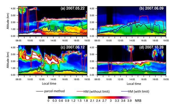
**Figure 8.** Time–height diagram of NRB (averaged every 11 minutes) on (**a**) 22 May; (**b**) 9 June; (**c**) 12 June; and (**d**) 28 October 2007. The CBLH calculated by the Haar wavelet method (HM) with (or without) the calculated CCL as an upper limit is marked by blue solid lines (or red solid lines), and the  $\Delta h$  used by the HM is set to 300 m based on the previous sensitivity test. The CBLH estimated by the parcel method is marked by black solid lines.
