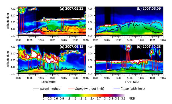
**Figure 7.** Time–height diagram of NRB (averaged every 11 min) on (**a**) 22 May; (**b**) 9 June; (**c**) 12 June; and (**d**) 28 October 2007. The CBLH calculated by the idealized backscatter method (*fitting*) with (or without) the calculated CCL as an upper limit is marked by blue solid lines (or red solid lines). The CBLH estimated by the parcel method is marked by black solid lines.
