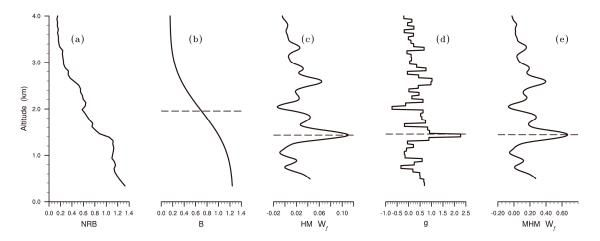
**Figure 1.** (a) Normalized Relative Backscatter (NRB) profile at 13:00 local time on July 23, 2007 and profiles of (b) fitted curve (*B*); (c) Haar wavelet coefficient (HM  $W_f$ ); (d) gradient (g); and (e) Mexican hat wavelet coefficient (MHM  $W_f$ ). The CBL (Convective Boundary Layer) tops from these profiles are shown as horizontal lines, and the parameter  $\Delta h$  used by the HM and MHM is set to 300 m.
