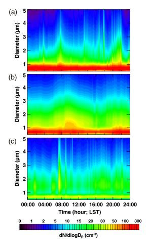
**Figure 6.** Same as Fig. 5 but for aerosol size distribution  $(dN / dlog D_p, 0.5 \, \mu m < D_p < 5 \, \mu m)$  in (a) Wuwei, (b) Zhangye, and (c) Dunhuang from 3 April to 16 May 2014. Note that data collected during the strong dust storm in Zhangye are excluded.
