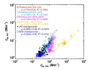
**Figure 11.** Scatter plot of aerosol absorption coefficients versus scattering coefficients from 3 April to 16 May 2014. The color symbols represent different atmospheric conditions during the dust field campaign.
