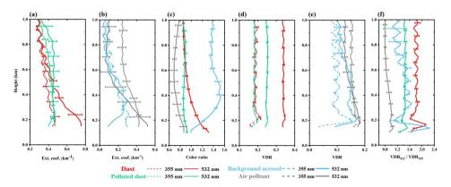
**Fig. 3.** Vertical profiles of extinction coefficients at 532 nm and 355 nm (a-b); color ratio (c); VDR at 532 nm and 355 nm (d-e) and VDR<sub>532</sub>/VDR<sub>355</sub> (f) from atmospheric aerosols observed by the lidar system for four aerosols.
