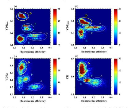
**Fig. 7.** Relationship between the fluorescence efficiency  $\eta$  and (a) VDR532, (b) VDR355, (c) VDR<sub>532</sub>/VDR<sub>355</sub>, (d) CR for air pollutants (A), dust (D), polluted dust (P) and background aerosol (B) over northwest China during April of 2014. The grid resolution is  $500 \times 500$ .
