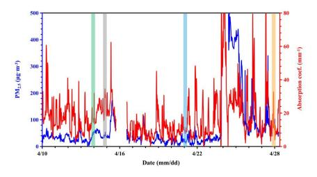
**Fig. 2.** Variations in  $PM_{2.5}$  and absorption coefficient near the ground surface during April 2014 at Linze. The shadows in blue represent background aerosol, yellow dust, green polluted dust, and gray air pollutants.
