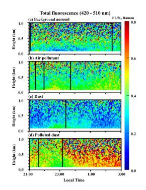
**Fig. 4.** Vertical structure of the total fluorescence signal between 420 and 510 nm for four aerosols: Background aerosols (a), Air pollutant (b), Dust (c) and Polluted dust (d).
