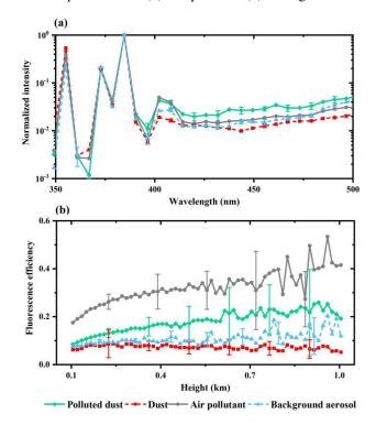
**Fig. 5.** (a) Normalised fluorescence spectra between 340-520 nm and vertical profiles of (b) fluorescence efficiency from atmospheric aerosols observed by the lidar system for four aerosols.
