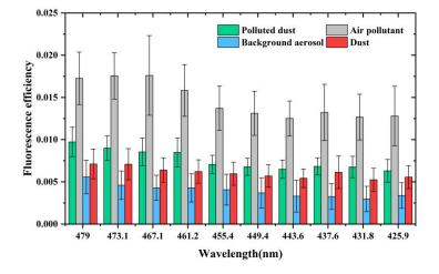
**Fig. 6.** Mean and standard deviation of fluorescence efficiency between 425.9 nm and 479 nm for four aerosols.
