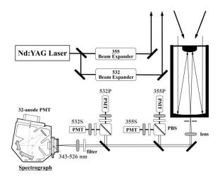
Fig. 1. Schematic diagram of the spectroscopic lidar system developed in this study.
